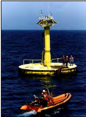
Figure 3-8a 10-meter Discus-shaped Hull Buoy
