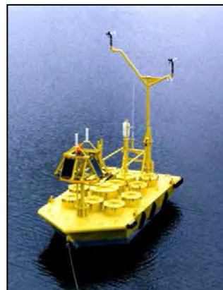
Figure 3-8b 6-meter Boat-shaped Hull Buoy
